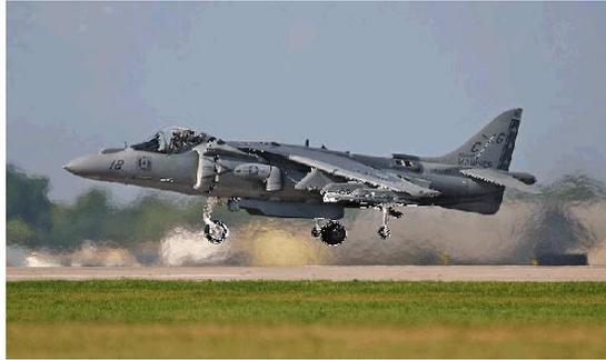
The Harrier Jump Jet, sometimes referred to as simply the "Harrier", is a British designed military jet aircraft capable of Vertical/Short Takeoff and Landing via thrust vectoring. The Harrier family is the only truly successful design of this type emerging from the various attempts in the 1960s.
